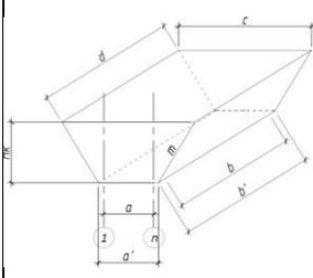
$a' = a + 2 \times (b\phi/2 + 0,7)$ $b' = b + 2 \times (b\phi/2 + 0,7)$ $c = a' + 2 \times Hk * m$ $d = b' + 2 \times Hk * m$ $Vk = [(a' \times b') + (c \times d) + (a' + c) \times (b' + d)] \phi$ | м <sup>3</sup> |        |                                                                                                                                |
